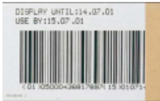
Bar code printed too close to edge of label.
